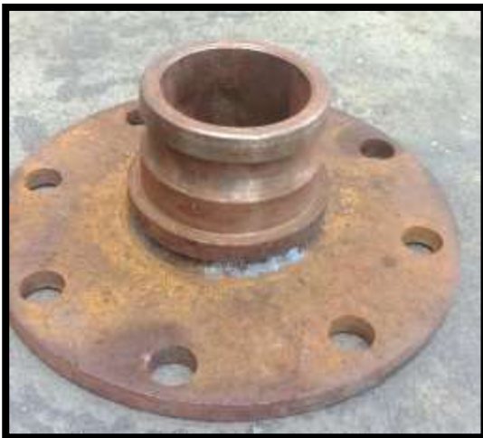
Picture 8 – Fuel Coupling (Type B) Male End: Image and Dimensions
