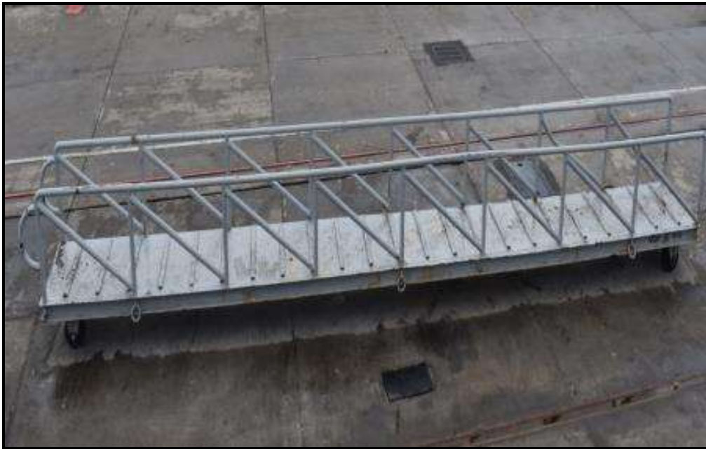
Picture 1 – Ship's Brow (Length - 40 feet with roller on both ends)
