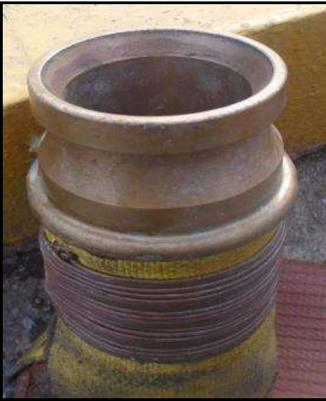
Picture 5 – Fresh Water Coupling Male End – Image and Dimensions
